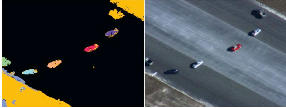
Figure 1. Left: an example of segmentation obtained by applying the tracking method [21]. Right: the corresponding video frame from the DARPA VIVID video set [25].
